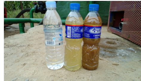
Oily Water (central), After Filtration (left), Concentrated Water (right)
